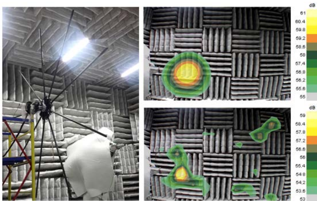
Figure 6. Localization of noise sources at frequency of 800 and 2000 Hz at jet velocity of M=0.5 .
