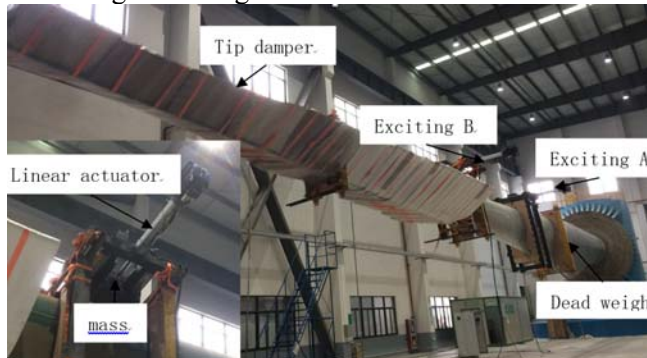
Fig.4(a) Horizontal dual-point exciter mounted on the blade
