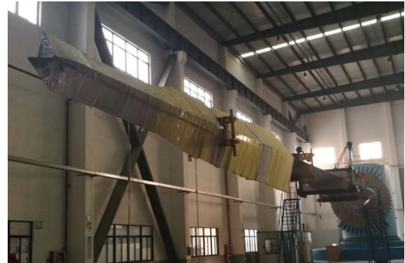
Fig.4(b) Vertical single-point exciter mounted on the blade
