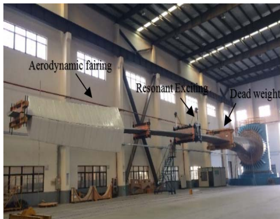
Figure 4. Aerodynamic fairing and blade mounted in flapwise direction
