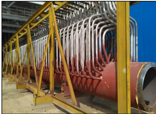
Figure 5. Photo of boiler pipe header
