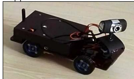
Figure 4. Photo of wireless magnetic crawler
