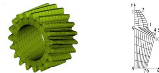
Fig.6 Overall arrangement form of gear mesh Fig.7 Right end of the single tooth mesh
