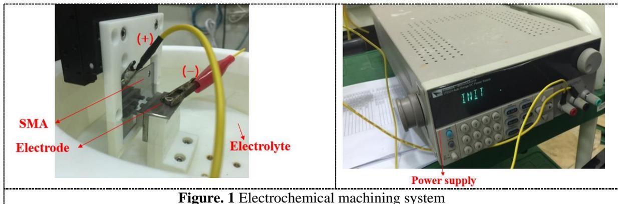
**Figure. 1** Electrochemical machining system
