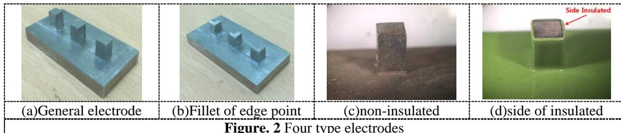
**Figure. 2** Four type electrodes
