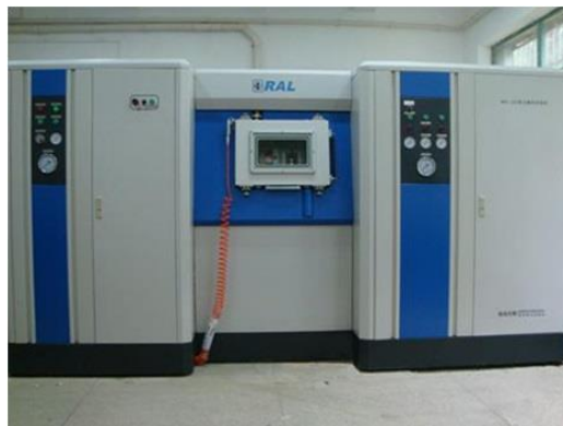
Figure 2. MMS-200 thermal-mechanical simulator
