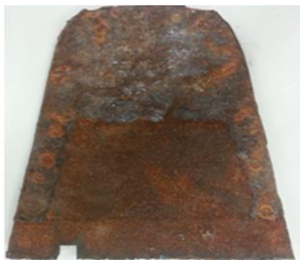
Figure 2: Hardfacing coverage of carbon steel blade using SMAW: (a) top view and (b) front view.
