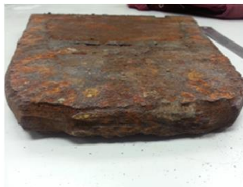
Figure 2: Hardfacing coverage of carbon steel blade using SMAW: (a) top view and (b) front view.
