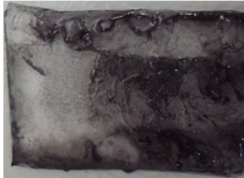
Figure 8: PDMS printing plate condition after being used with CNT solvent base ink
