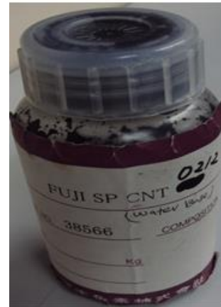
Figure 4: Carbon Nanotube (CNT) water base ink
