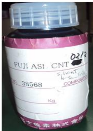
Figure 3: Carbon Nanotube (CNT) solvent base ink
