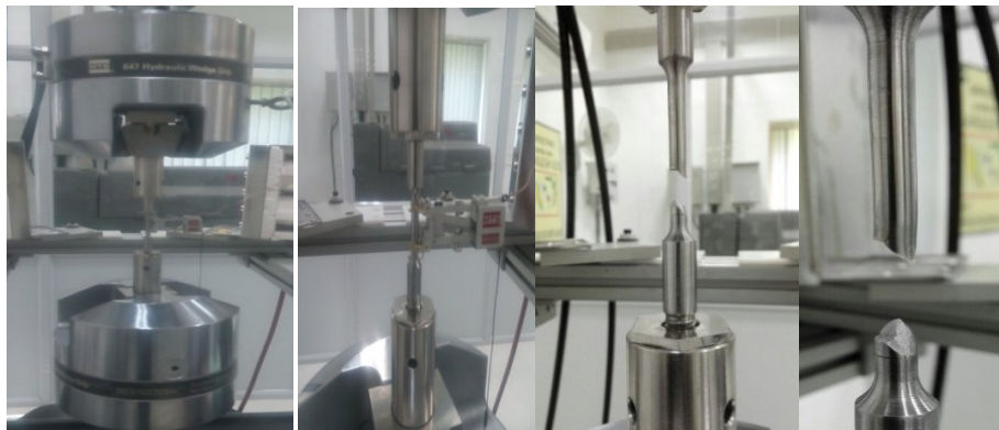
Figure 3. Specimen for Low Cycle Fatigue Test mounted on MTS
