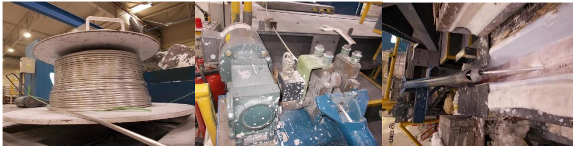
Figure 2. Supply system of the Al-Ti-B master alloy (Source: UAC Europe SRL)
