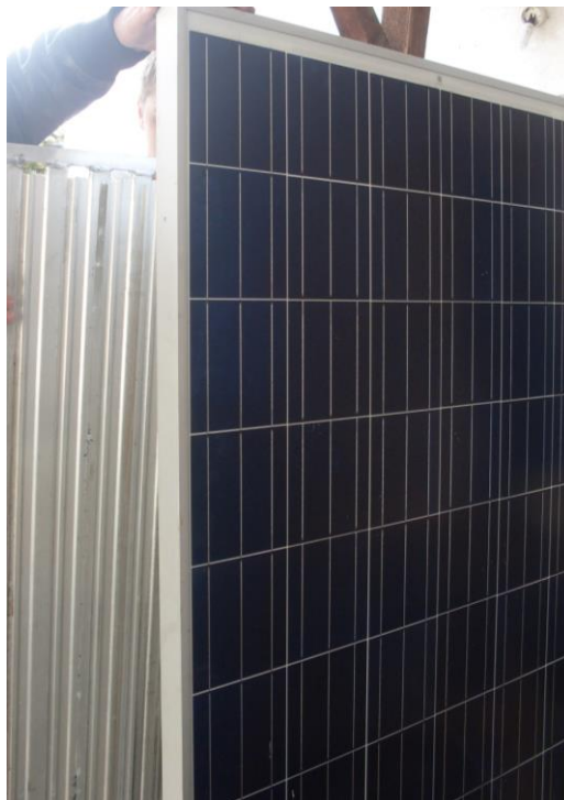
Figure 3. PV and thermal part of solar panel before finishing
