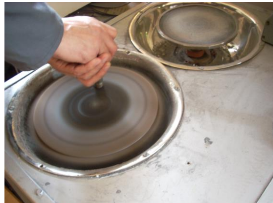
Figure 7. Equipment for preparing metallographic samples
