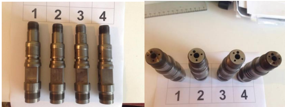
Figure 1. The batch of the studied injector bodies
