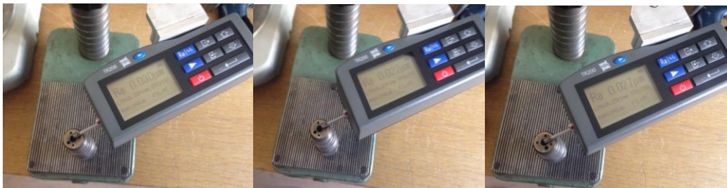
Figure 2. Measuring the roughness of the injector body
