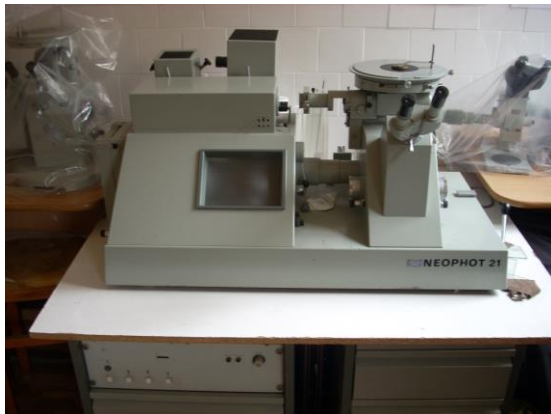
Figure 6. Metallographic microscope
