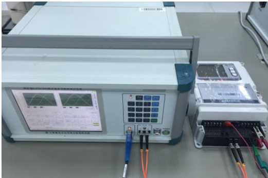
Figure 3. Standard digital power source and the meter being tested
