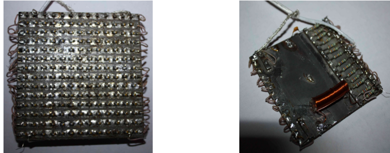
Figure 6. The prototype of the microstrip lattice with nonlinear loads: front side (left) and back side (right).
