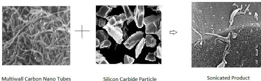
Figure 3. Mixing of multi wall carbon nano tube with silicon carbide particle and the resultant product of sonication
