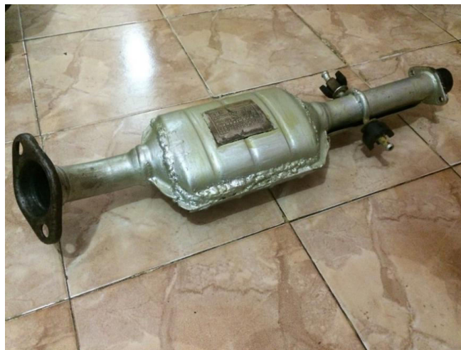
Figure 3. Assembled Catalytic Converter
