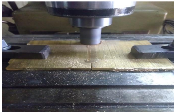
Figure 1. Friction stir welding
