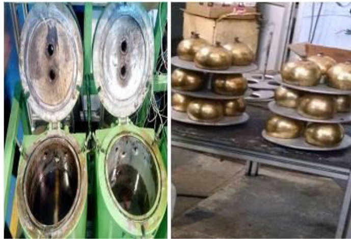
Figure 2. PCM tank & fixed bed arrangement
