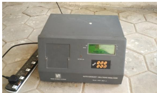
Figure 2. NETEL Auto exhaust / multi gas analyzer
