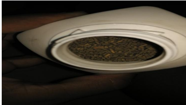
Figure 4. Molecular sieve 5A crystals of 1.5mm
