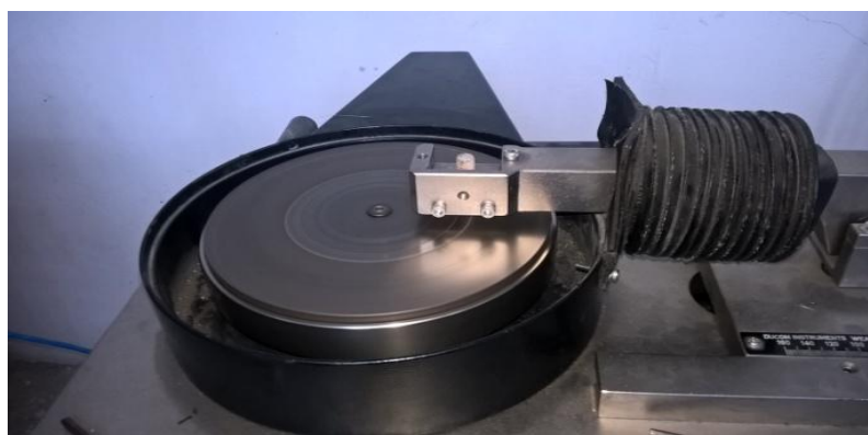
Figure 4. Pin on disc experiment set up.
