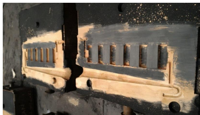
Figure 2. Visualization of the mould after the application of double-layer coating
