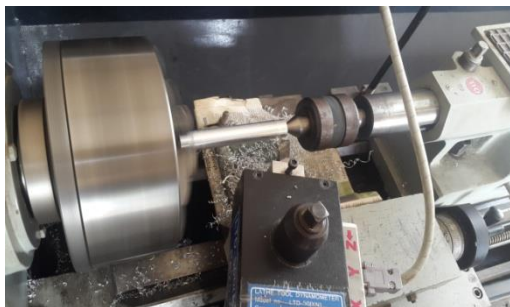
Figure 1. Lathe Tool Dynamometer
