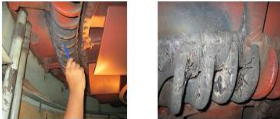
Figure 1. Short circuit W-phase stator generator
