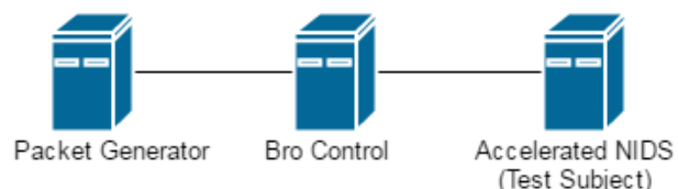
Figure 3: AMD Environment Testing Network Architecture
