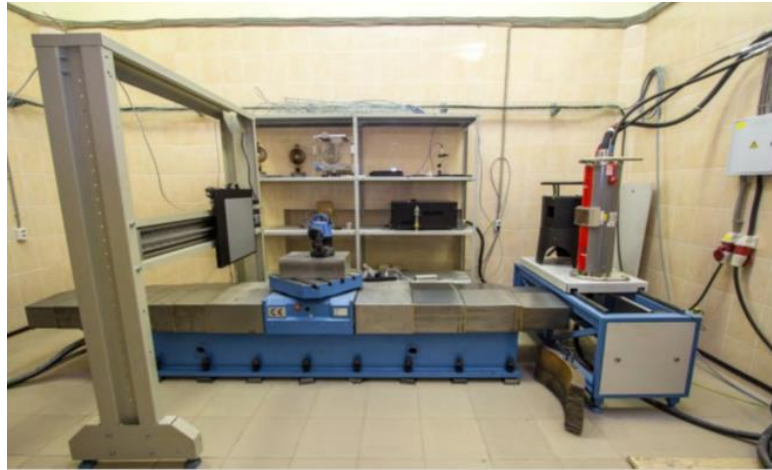
Figure 1. Betatron tomography system.
