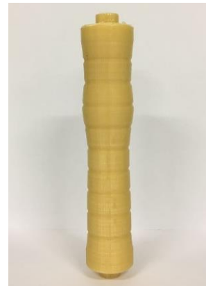
Figure 4. Sacrificial water solubility core manufactured by FDM.
