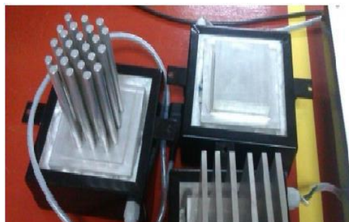
Figure 3. Designs of heat sink, flat plate, rectangular fin and circular tube fin.
