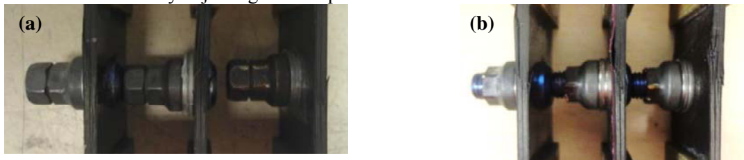
Figure 9. FHC test failure mode. (a)30% vacuum compaction, (b)100% vacuum compaction.
