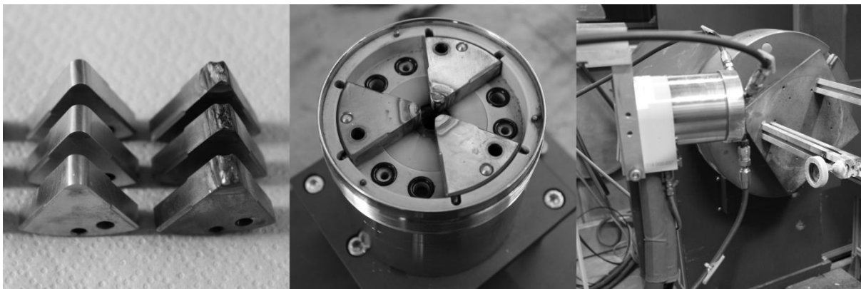
Figure 4. New and worn electrodes, electrode setup in the plasma spray gun and spray gun setup.
