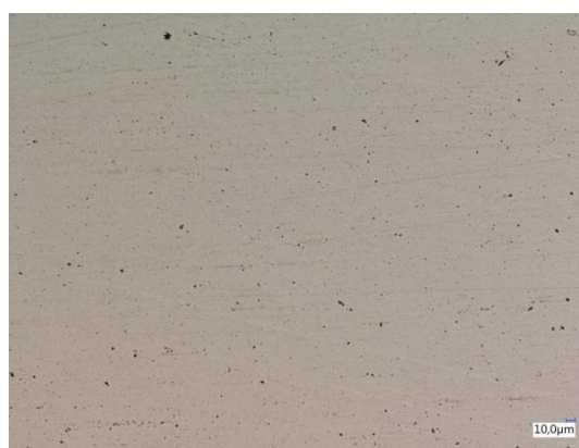
Figure 3. Crackfree layer, 3mA/cm 2 , 1 µm.
