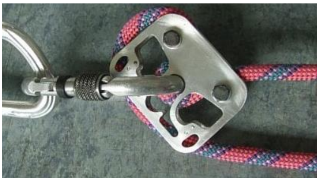
Figure 1. The developed belay device attached to an HMS carabiner and rigged with a climbing rope. The “control” rope can be seen at the bottom and the “life” rope at the top of the image. The control rope force introduced by the operator’s hand is amplified by the device, allowing the control of the life rope force.
