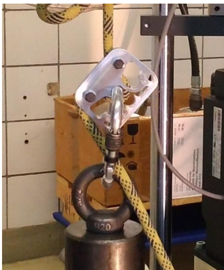
Figure 5. The belay device as it was tensioned during the pull test: The device attached to the tension testing machine with a carabiner, the life rope going upward and the control rope leaving the device at an angle of 30°.
