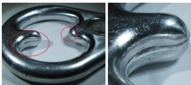
Figure 3. Burrs on the edges of the Bat Brake by Edelrid, where the excess material from drop forging was presumably removed by stamping.
