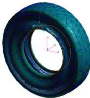
Figure 3. Tyre FE model
