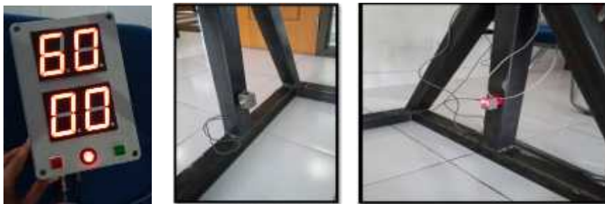
Figure 5. The series of infrared sensors on the bottom of the pole and LED box
