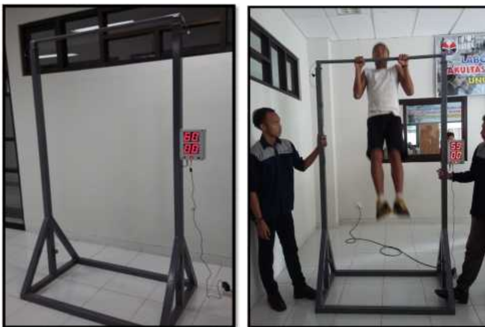
Figure 4. Prototype measuring instrument digital motion pull ups
