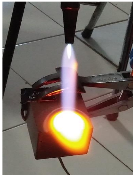
Figure 3. Fire resistance measurement on the surface of the composite
