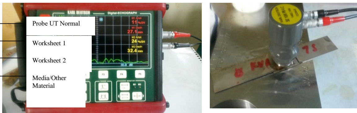
Figure 2.4 Identification Quality of Spot Welding used Non Destructive Test (NDT)-UT
