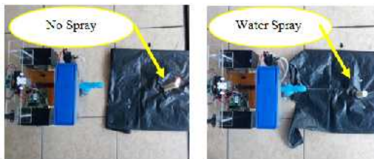
Figure 3. Water pump test (a) without and (b) with water spray
