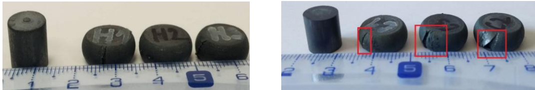
Figure 3. Specimens of TiNb alloys after the isothermal compression test: a) hydrogen non-charged, b) hydrogen charged (cracking in red boxes).
