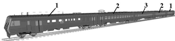
Figure 1. The solid-state computer model of the electric train: 1 – 'head car' subsystem; 2 – 'trailer' subsystem; 3 – 'powered car' subsystem.
