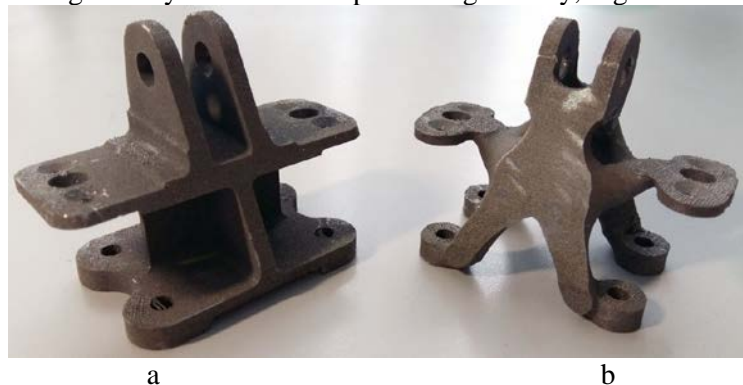
Figure 4. The parts produced with the SLM method by Aviadvigatel JCS: a – initial geometry; b – optimal geometry.
