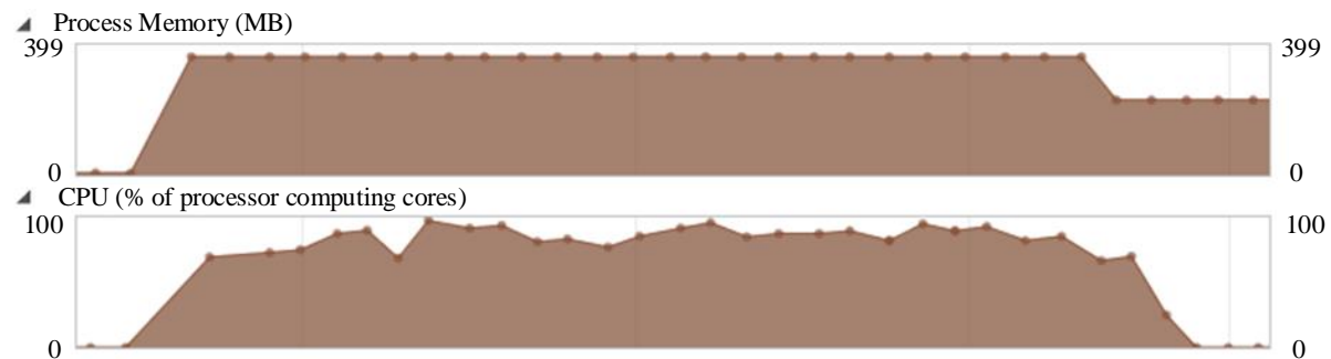
Figure 4. Memory usage and CPU utilization as functions of time, after optimization of memory allocation.
