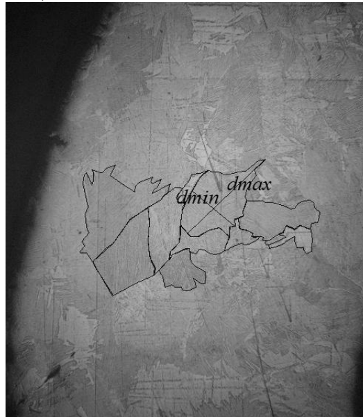
Figure 1. The microstructure of a sample annealed for 5 h, and the grain selection and size measurement pattern.
