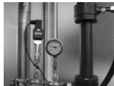
Figure 13. The pressure transducer and manometer below piston.
