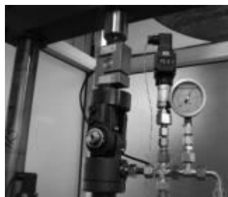
Figure 12. The pressure transducer and manometer above piston.
