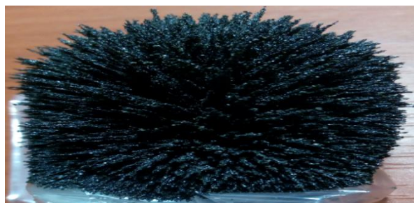
Figure 1. Iron sand attracted to the permanent magnet.
