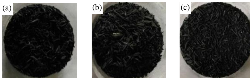
Figure 1. Carbon resulting from pyrolysis of rice husk at (a) 300 °C (b) 350 °C (c) 400 °C
