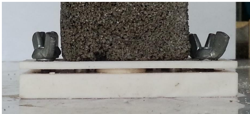
Figure 1. Device Used for Compression Set Test
