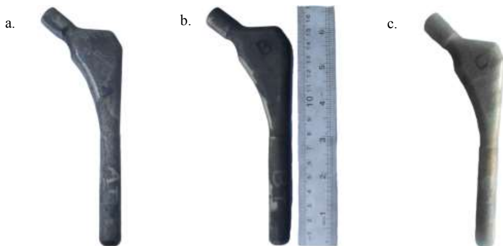
Figure 2. As-cast femoral stems without the gating system (a) first design (b) second design (c) third design
