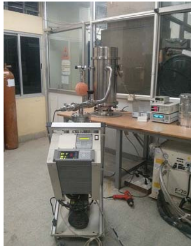
Figure 7. Photograph of the cryosorption pump with integrated with AVS procedure
