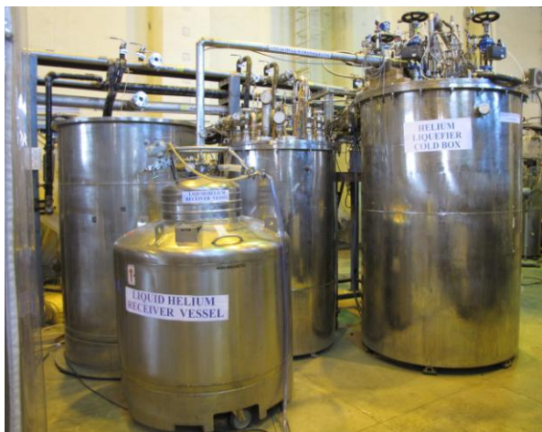
Figure 4. Developed helium refrigeration/liquefaction system
