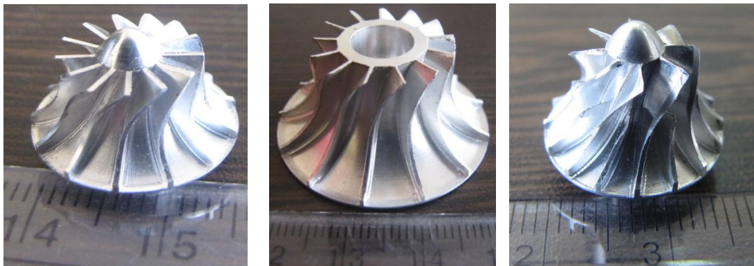
Figure 2. Photographs of the turboexpander wheels used in the developed system
