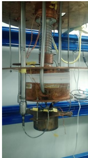
Figure 2. Assembled refrigeration cryostat.
